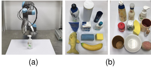
Fig. 10. Real setting of our robotic grasping experiments. (a) Robotic grasping experiment setup with HIT-DLR II Hand and UR5 robotic arm. (b) Objects used in our robotic experiments. Left part shows similar objects, right part shows novel objects.
